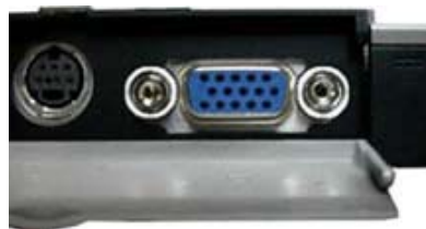
Fig. 32 Removing VGA port screws
